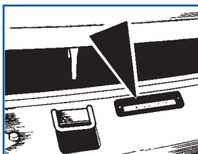
The Commission Number is stamped on a plate secured to the bonnet lock platform.
